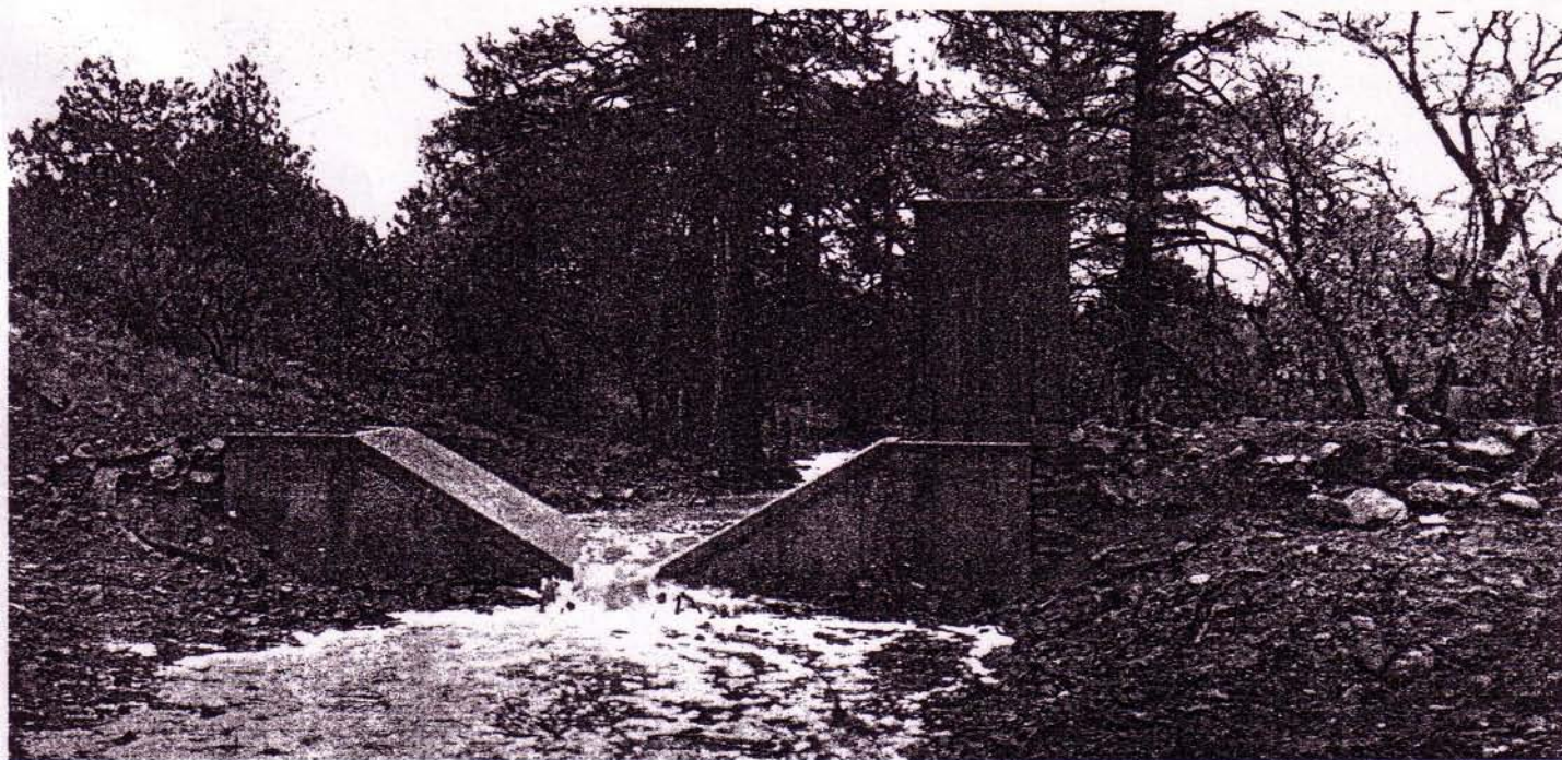
Figure 19.—Water flowing through measuring flume. The trees in this study watershed are mainly ponderosa pine. The surrounding soils are of the Brolliar series.
